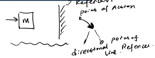
Oriented branch → Direction is assigned using an arrowhead → Positive direction of power flow → "Into" element at point of action, and "out of" element at point of reference (exception: "source") → Arrowhead of branch is pointed toward point of reference (exception: T-type source)
