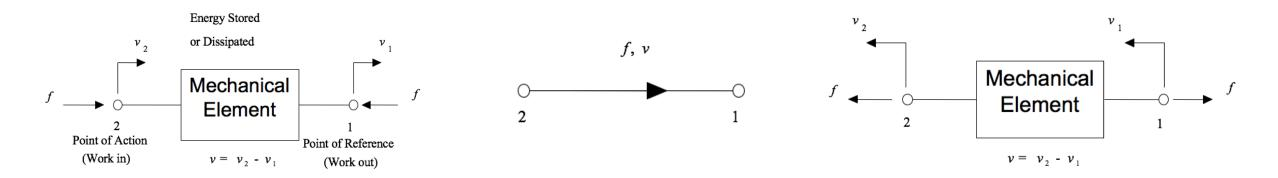
**Note:** Reversing the directions of both f and v won't affect power flow direction (See (a) and (c); Convention (a) is preferred
